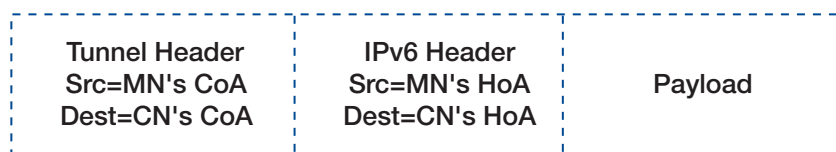
Figure 2.8.3: The IPv6 headers in E2T tunneled packets
